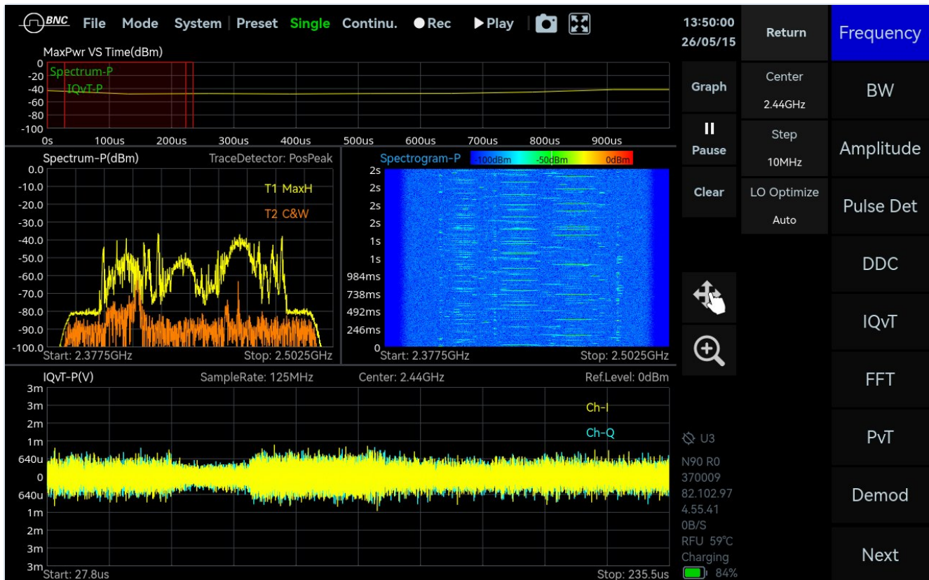
Figure 6. One acquisition presented four ways at once: power against time, max-hold and clear-write spectra, a two-second spectrogram, and I and Q across a 208 microsecond window with a sample-rate field reading 125 MHz. The span reads 2.3775 to 2.5025 GHz, which is 125 MHz, the sample rate rather than the usable 100 MHz, and that gap is the convention section 6 warns about visible as a setting. Read the spectrogram pane against the buffer arithmetic rather than past it: it covers two seconds, far longer than the 0.26 s the buffer holds at this rate, so the spectrogram is a live rolling display and not a view of one buffered acquisition. The IQ pane below it is the burst case of the table above. MEASURED
